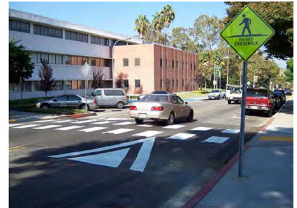
Figure 3.14.2. Typical Raised Crosswalk Application (Source: Jeff Guiden)
